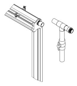
Last step Glue Main body, transition piece together, mount the bracket onto supporting wall and close the system with the old endcap.
