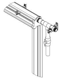
Replace the Endcap with the transition piece and glue assemble the traps main body as shown below.
