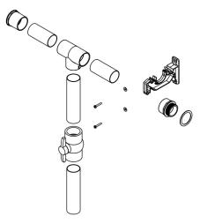
After the glue is cured, dry fit the assembly, including the pipe support bracket. Mark your drilling positions for the bracket as needed
