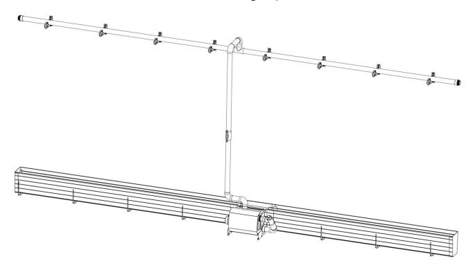
Use the Pad Guide Coupler to connect them over the whole length. For closing the Pad Guide Coupler push slider to right and clip in the left Pad Guide.
