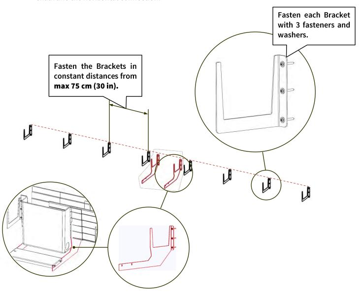
The Supply Unit is already pre-assembled. The Brackets of the Supply Unit must also been fasted in desired position.
